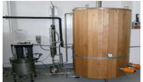
Heat extracts the sugars from the malt in a timber encased vat before the beer is transferred to the uninsulated cool tank to finish brewing
